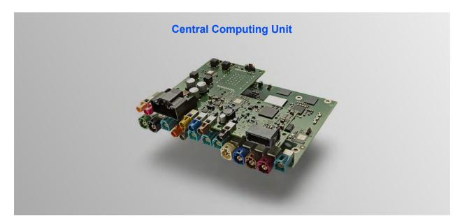
LeanCore can manage two displays of up to 12.3 inches and two cameras – including rearview and driver monitoring systems – and delivers high-performance processing and excellent adaptability on mature technical foundations. Phone mirroring via Android Auto™ and Apple CarPlay™ is also supported.
