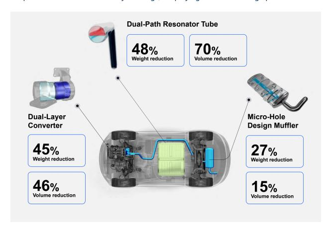
Together with thinner-gauge stainless steel, LeanExhaust's innovations contribute to a 16 kg weight reduction compared to conventional exhaust systems, while exceeding or matching emissions-control and noise-reduction performance.
