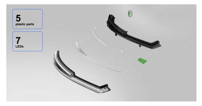
Multiple functions – including the turn indicator and taillight – are also consolidated onto a single electronic board. This MCU-free hardware approach is future-ready and fully compatible with the centralized domain and zonal controllers of SDVs, ensuring seamless compatibility with next-generation electronic architectures.
