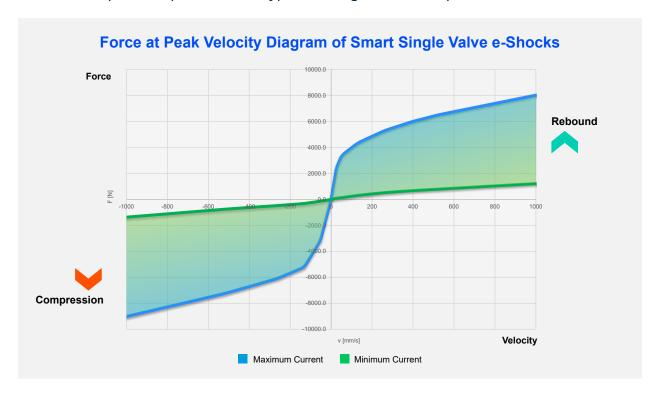
Optimizing the **tri-tube internal architecture** of the Smart Single Valve e-Shocks is key, with Marelli engineers using the piston area – rather than the piston rod – to generate compression damping. Depending on the application, a **100-200% improvement in compression performance** is achievable.
