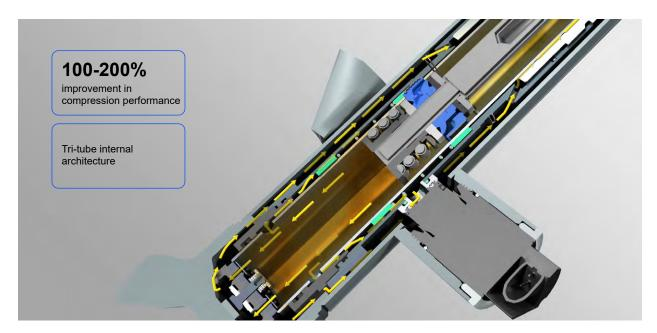
Only a software update is required to upgrade from Marelli's entry-level Single Valve e-Shocks to Smart Single Valve e-Shocks. The same single electrical connector is retained, while the sensor set, wiring harness, ECU and four external electro-valves are identical.
