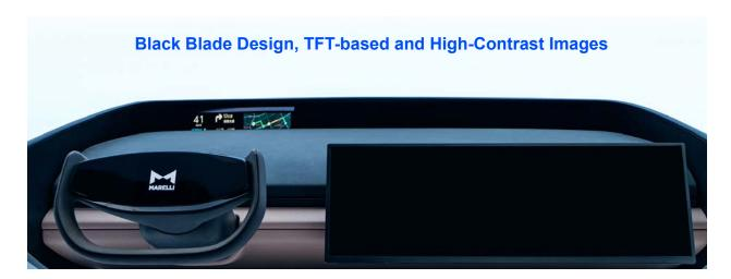
Dual-depth projection enables the prioritization of primary and secondary information – including Augmented Reality elements – at different depths on the windshield, making information easier for drivers to process.
